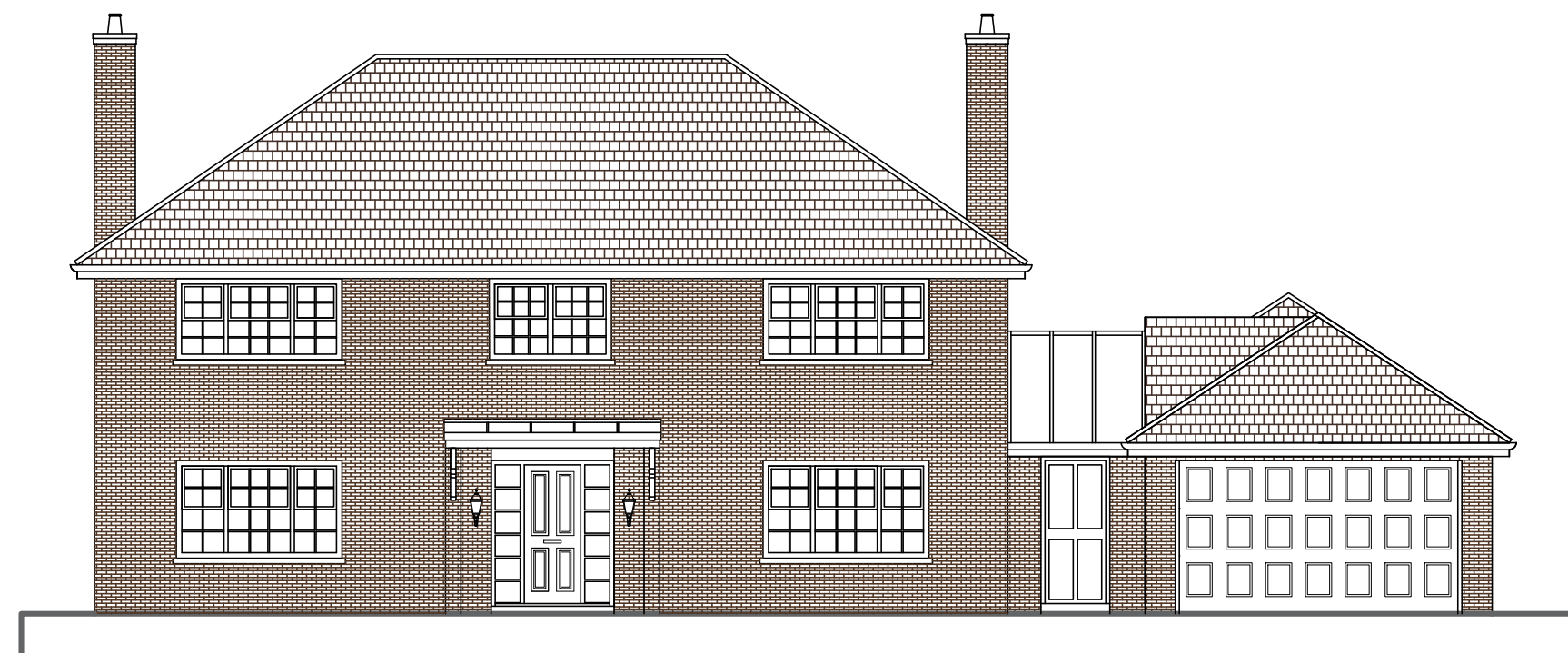
EXISTING FRONT ELEVATION
