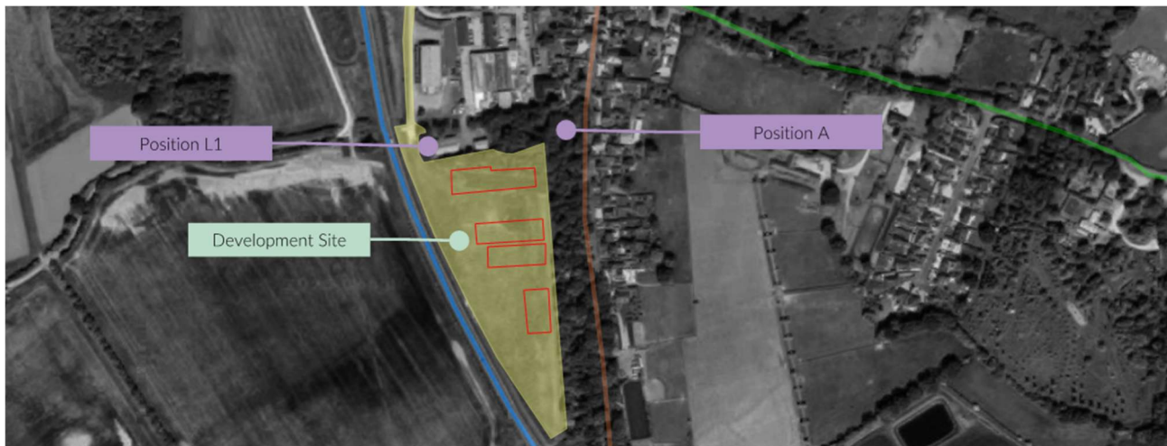
Figure 2: Satellite image showing the acoustic survey measurement locations.
