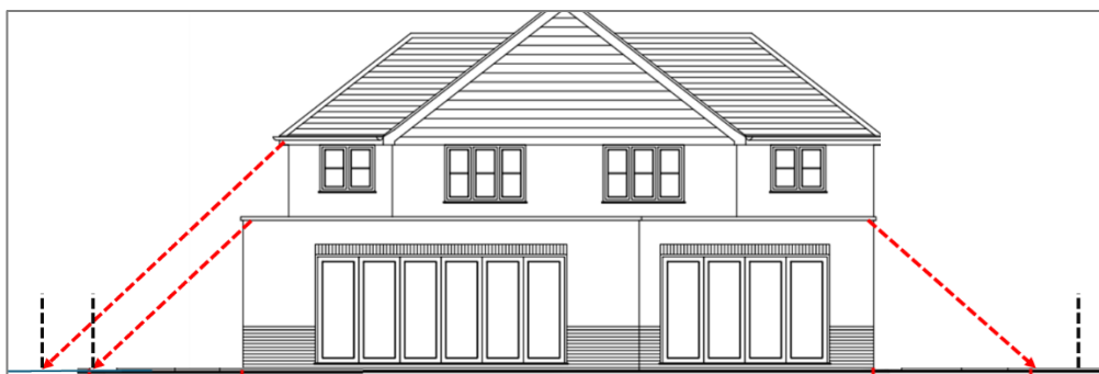
Figure 2 Vertical 45-degree angle test
