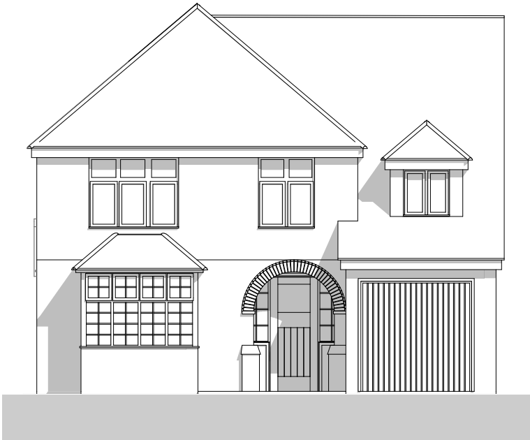
1:100 Existing Front Elevation
