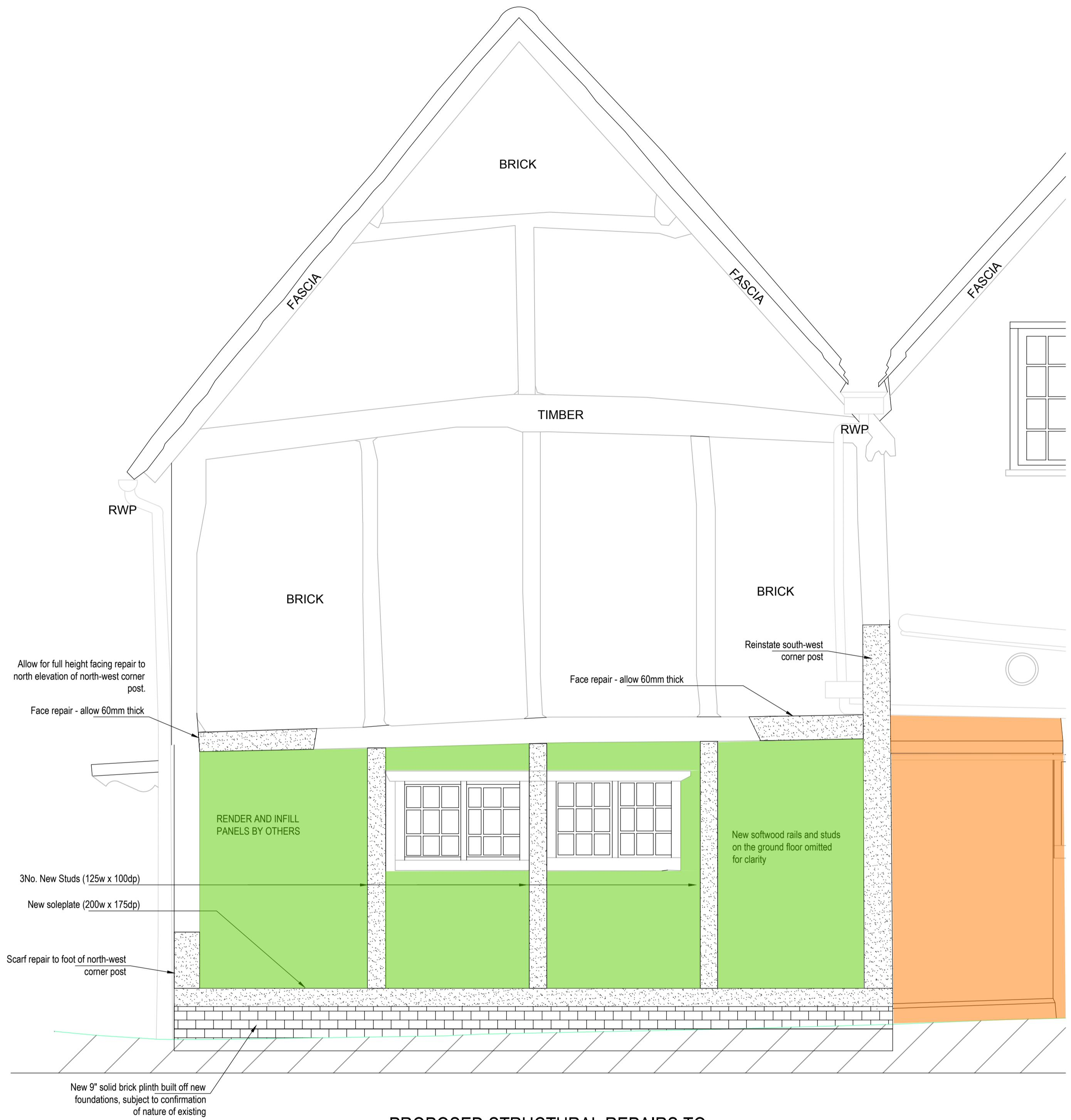
PROPOSED STRUCTURAL REPAIRS TO
