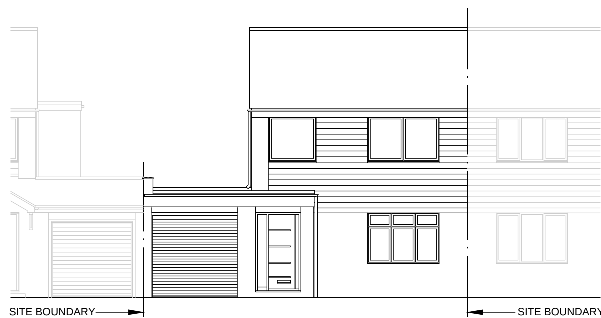
EXISTING EAST-FRONT ELEVATION
