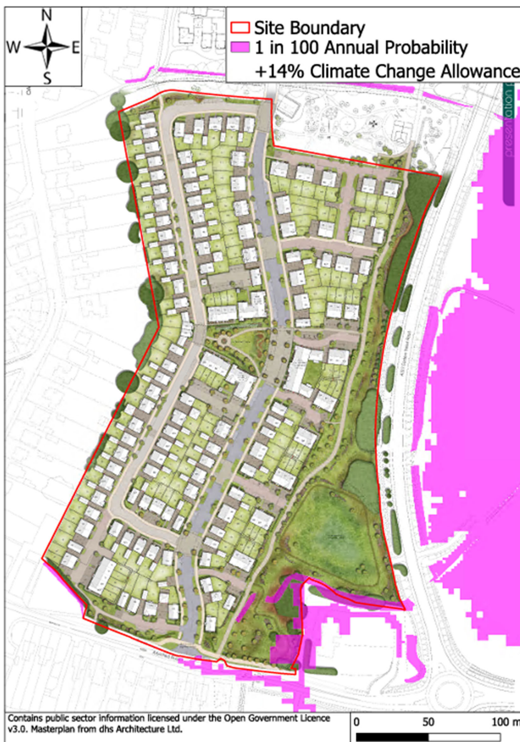
Figure 4: May 2026 Flood Modelling: 1 in 100 annual probability with climate change (design event)-on Masterplan
