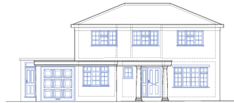
EXISTING FRONT ELEVATION
