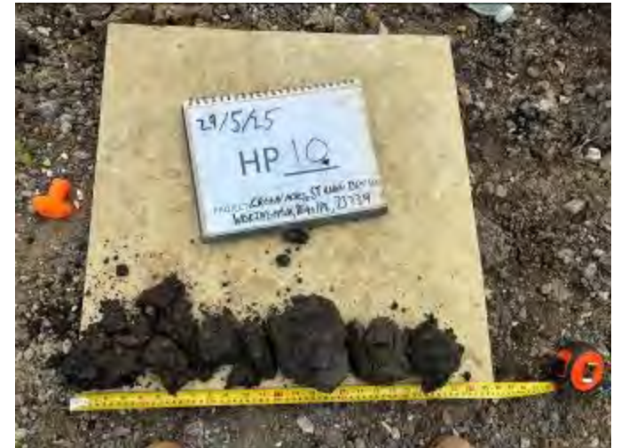
HP10 Topsoil and Subsoil Arisings
