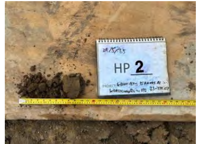
HP2 Topsoil and Subsoil Arisings
