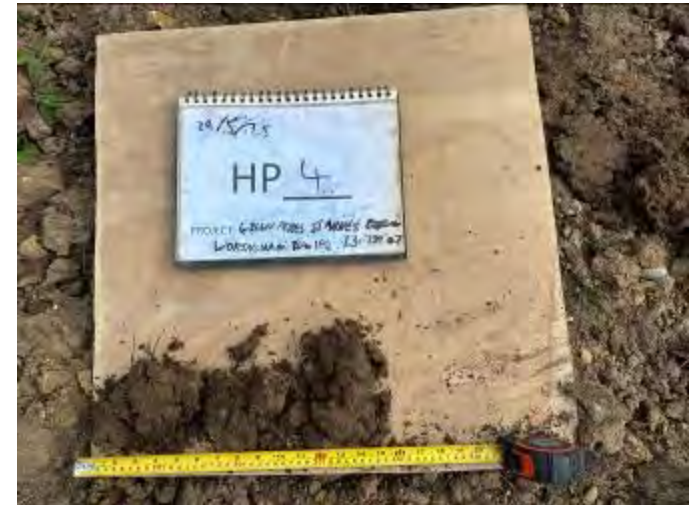
HP4 Topsoil and Subsoil Arisings
