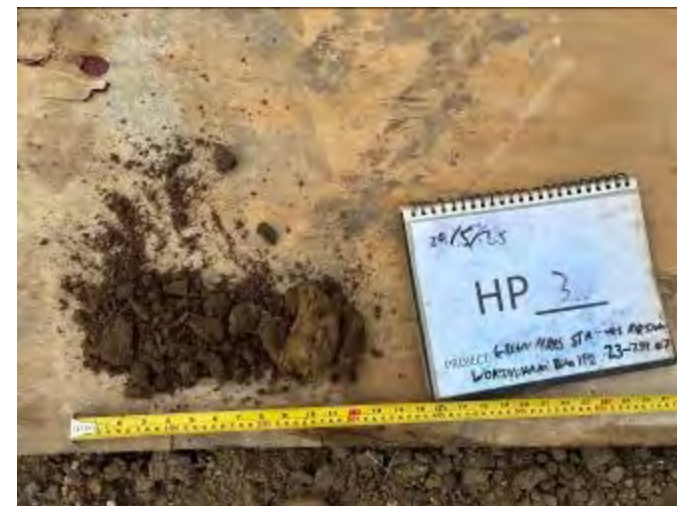
HP3 Topsoil and Subsoil Arisings
