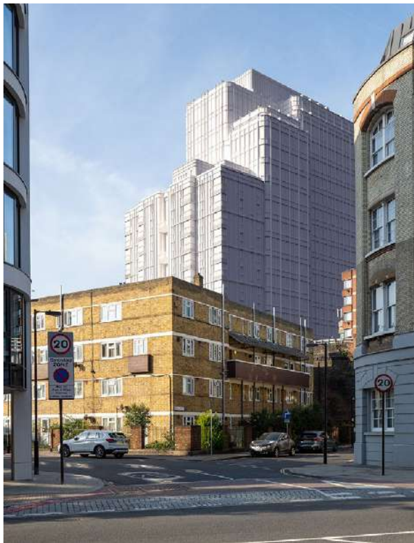
AVR2 (Clay) Explaining architectural form This example — a lit render in a uniform opaque ‘clay’ material. Masked out where occluded.
