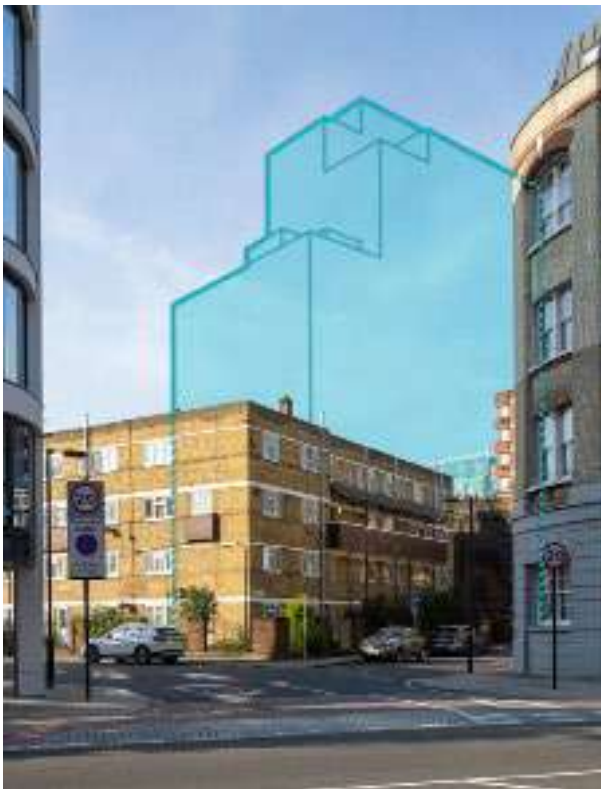
AVR1 (Wireline) Confirming degree of visibility This example — a ‘wireline’ (outline and edges) with a translucent fill. Dashed-line and no fill where occluded.
