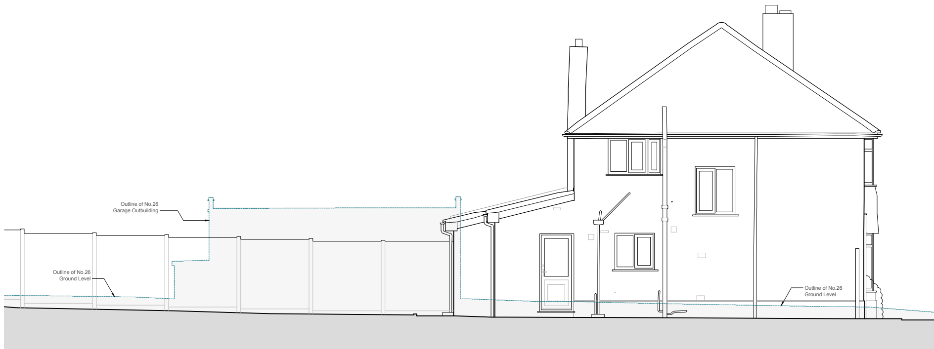
EXISTING WEST ELEVATION
