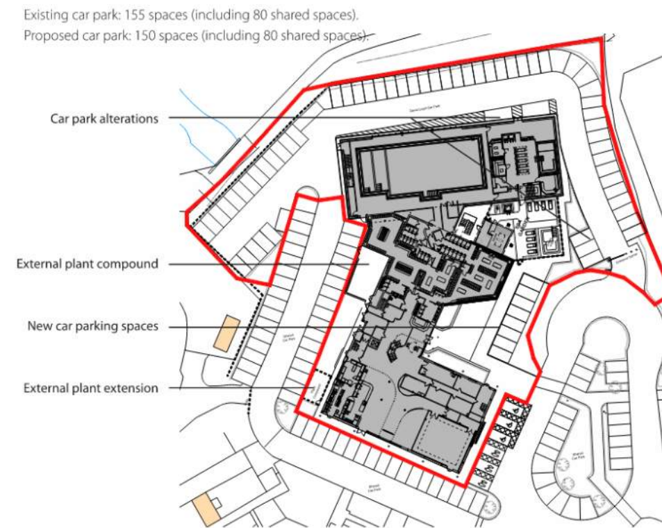
Figure 5: External plant and car park alterations
