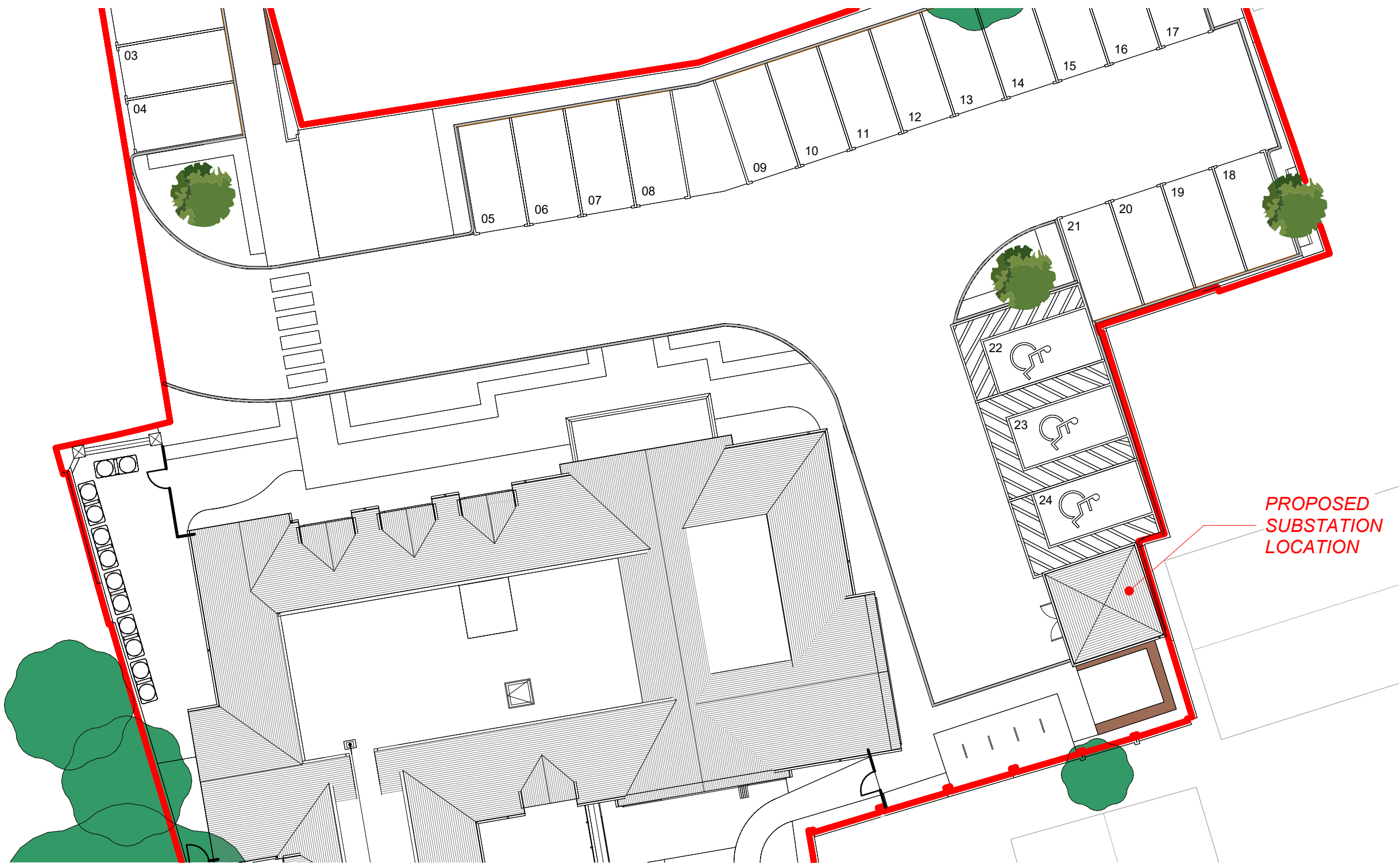
Substation - Car Park Plan 1 : 200
