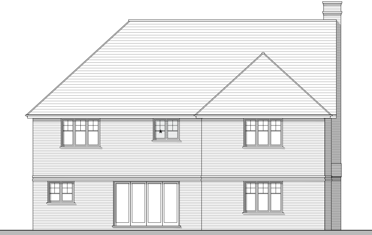
Rear Elevation ★ Denotes obscure glazing
