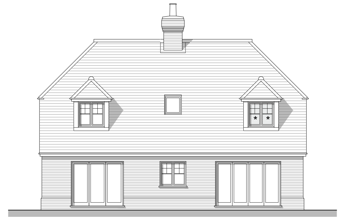
Rear Elevation ★ Denotes obscure glazing
