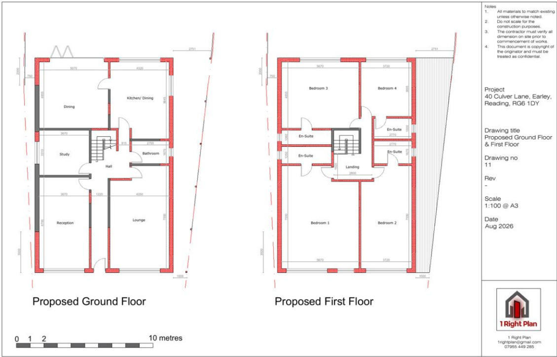
Figure 6: Proposed ground and first floor plans (drawing no. 11).
