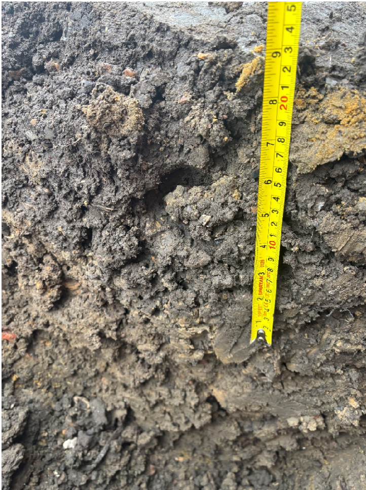
Inspection Pit excavated by client in Plot 133 showing 220mm of topsoil(client-provided photograph)
