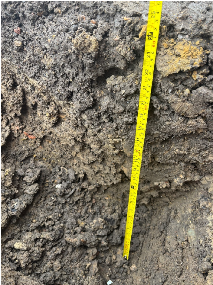
Inspection Pit excavated by client in Plot 141 showing 630mm of clean cover and 160mm of topsoil (client-provided photograph)
