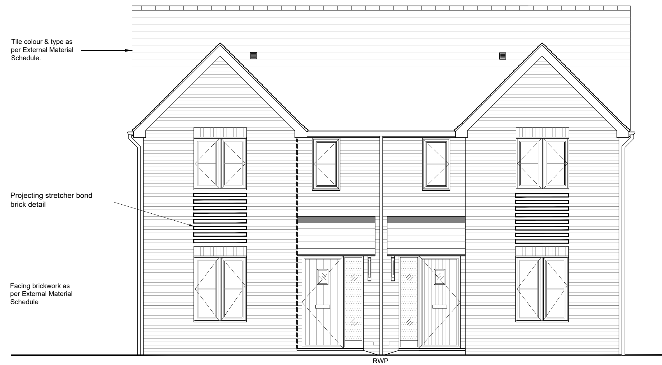
FRONT ELEVATION SCALE 1:50
