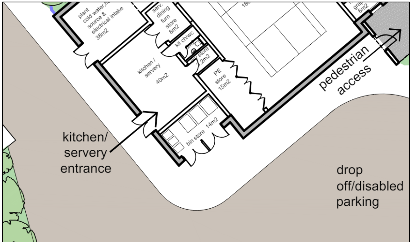
Figure 4.1: Waste Storage within the proposed development
