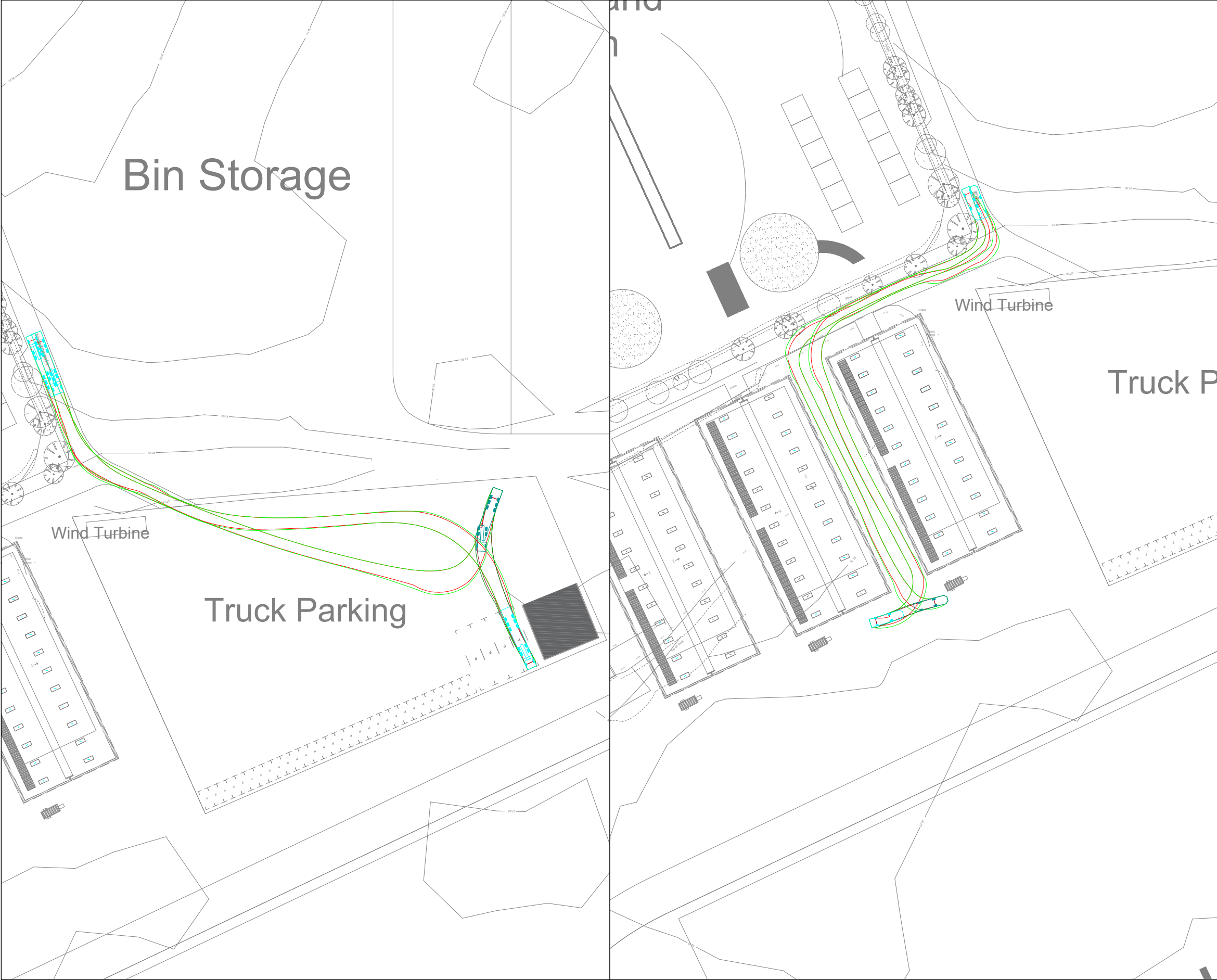
16.5M ARTICULATED VEHICLE TRACKING 1:500
