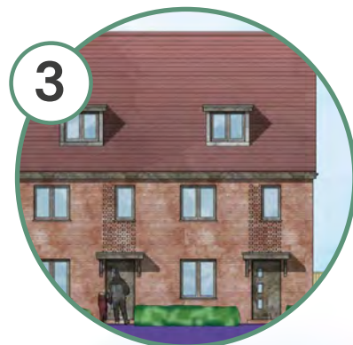
Extruded flemish brick detailing
