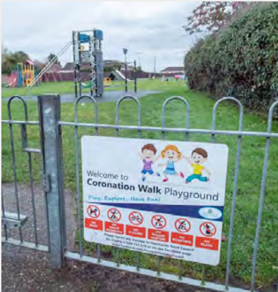
Powder coated aluminium sheet to be fixed to bowtop railing Dimension: min. 500mm x 400mm Example shown: Fitzpatrick Woolmer n'Viro graphic panel
