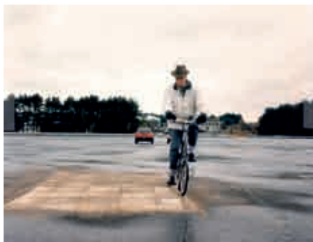
Fig. 2.7 Cyclist involved in track trials of humps
