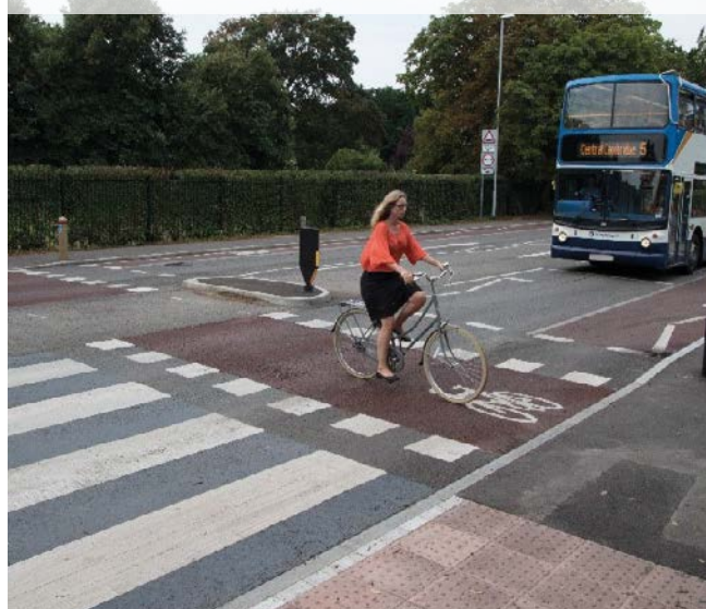
Figure 10.4: Parallel crossing with refuge
