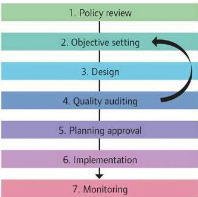
Figure 14.9: Highways, overall improvements process
