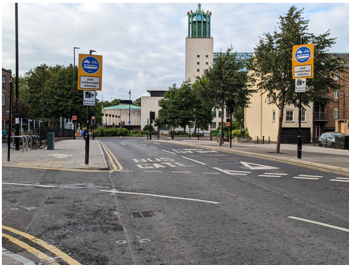
(Figure 24: bus gate with authorised vehicles permitted and camera enforcement)
