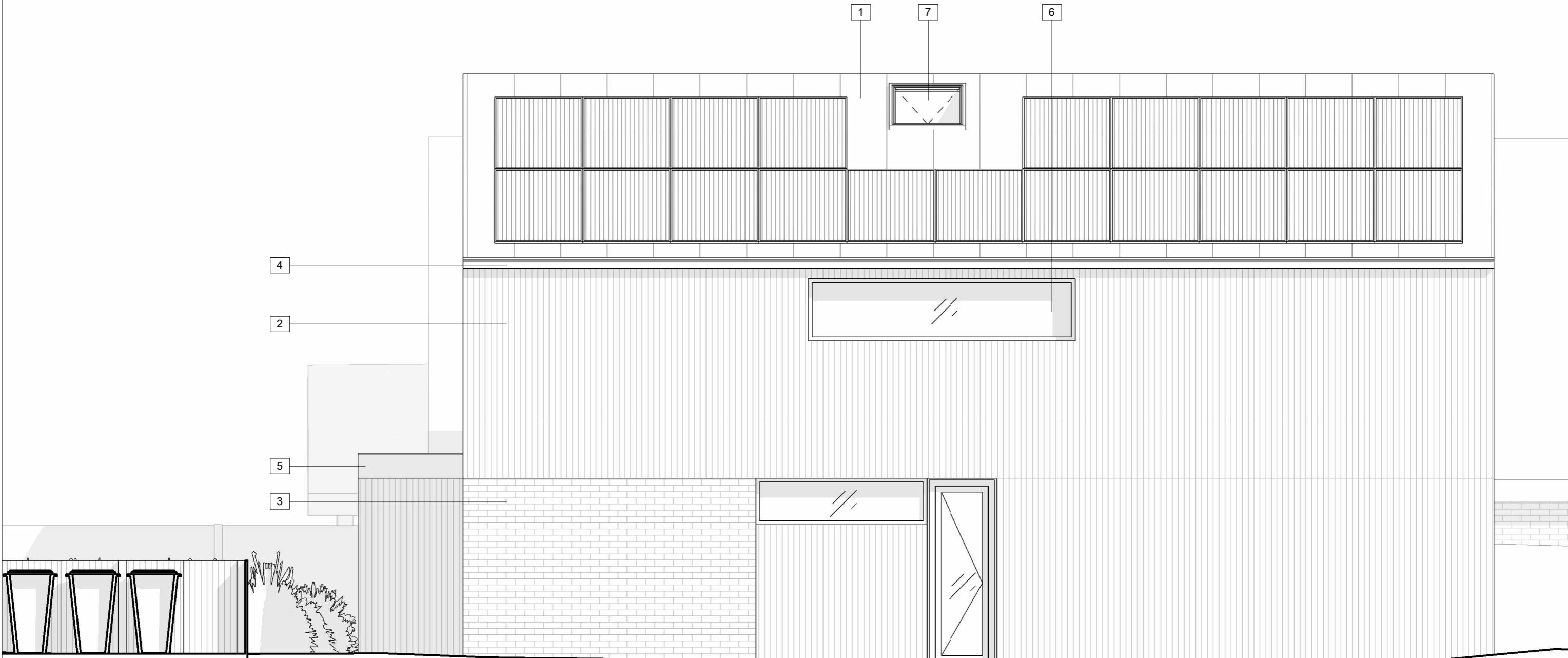
1 STANDING SEAM METAL ROOF WITH INSET PV ARRAY
