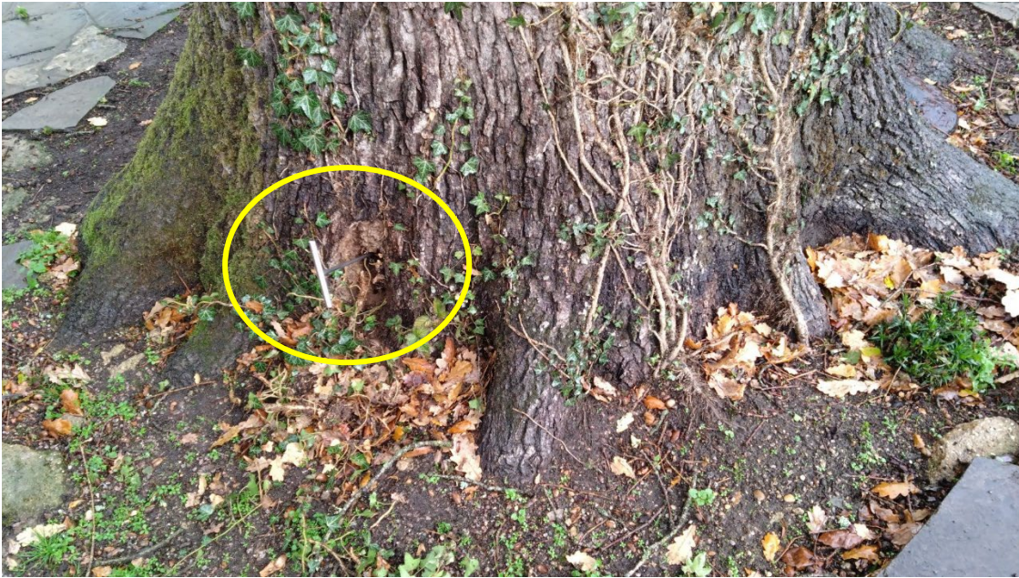
60cm long steel probe inserted into void on the west side.
