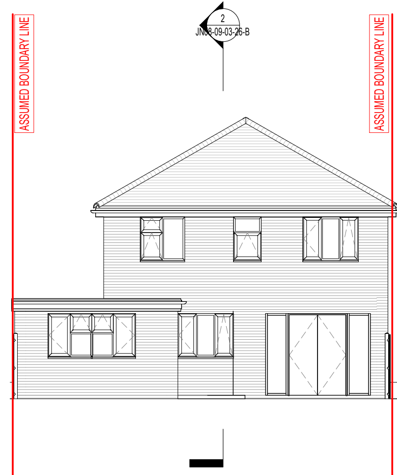
5 Existing rear elevation 1:100
