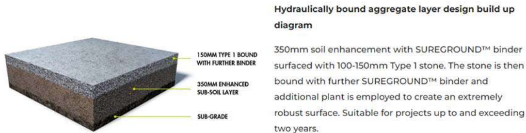
Figure 8: Western Hydraulically bound aggregate layer Haul Road
