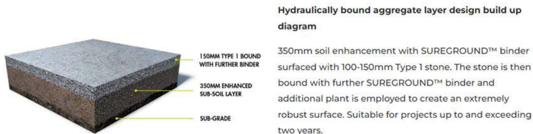
Figure 8: Western Hydraulically bound aggregate layer Haul Road
