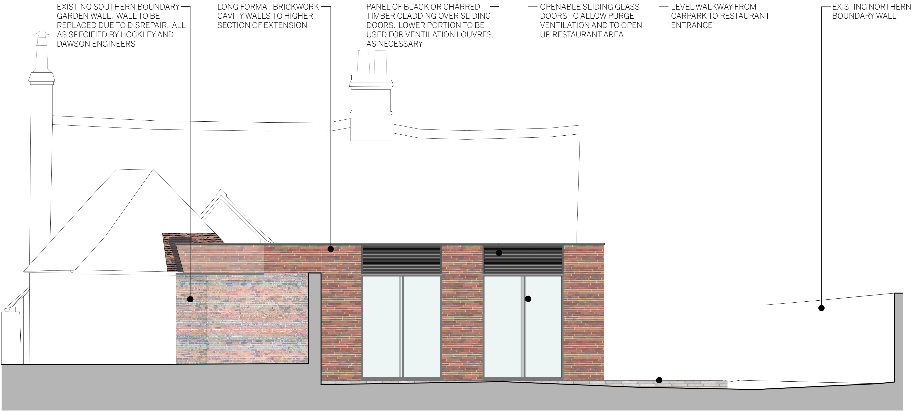
PROPOSED EAST ELEVATION(PERGOLA REMOVED)
