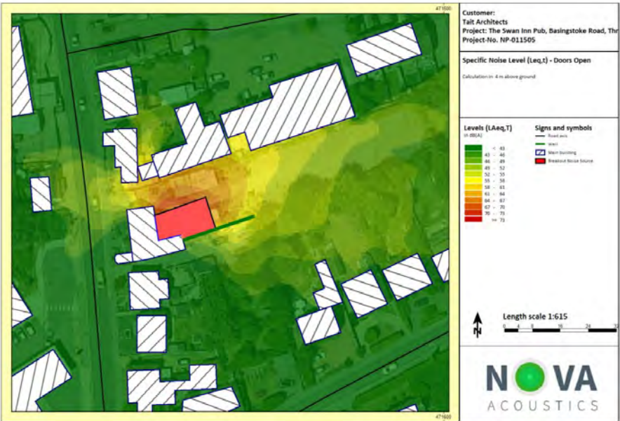
Fig 2.3 Noise assessment model showing likely noise breakout with restaurant doors open
