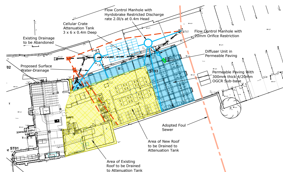
Fig 4.2 Proposed drainage strategy plan by Lanmor Consultant Engineers
