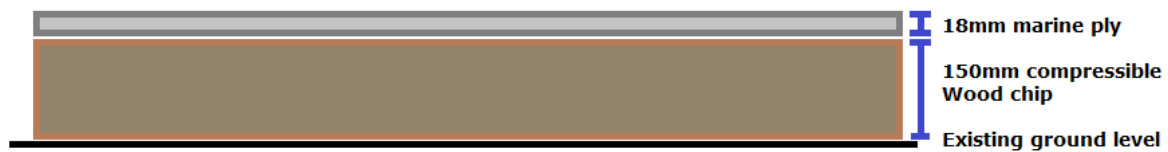
Above: ground protection make-up
