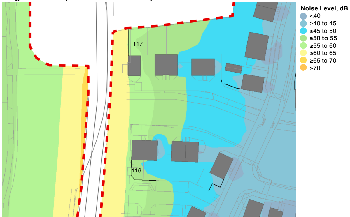
Image 6: Most exposed external amenity areas
