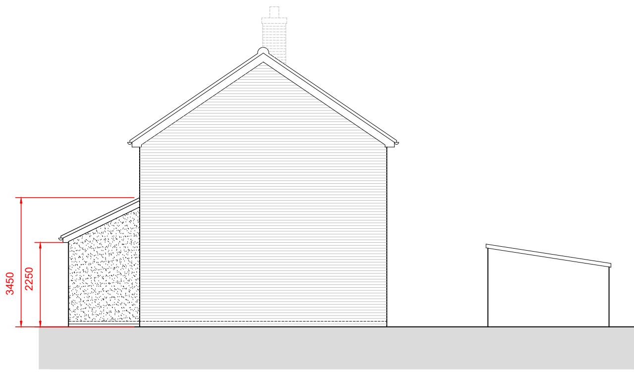
PROPOSED EAST ELEVATION SCALE 1 : 100
