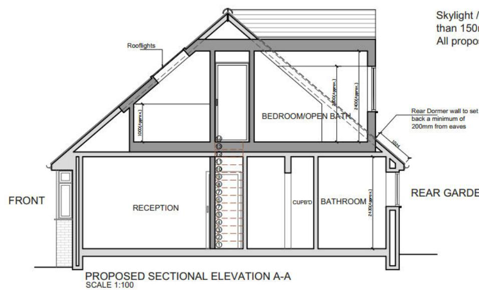
Skylight / Roof windows to not project more than 150mm from the roof slope
