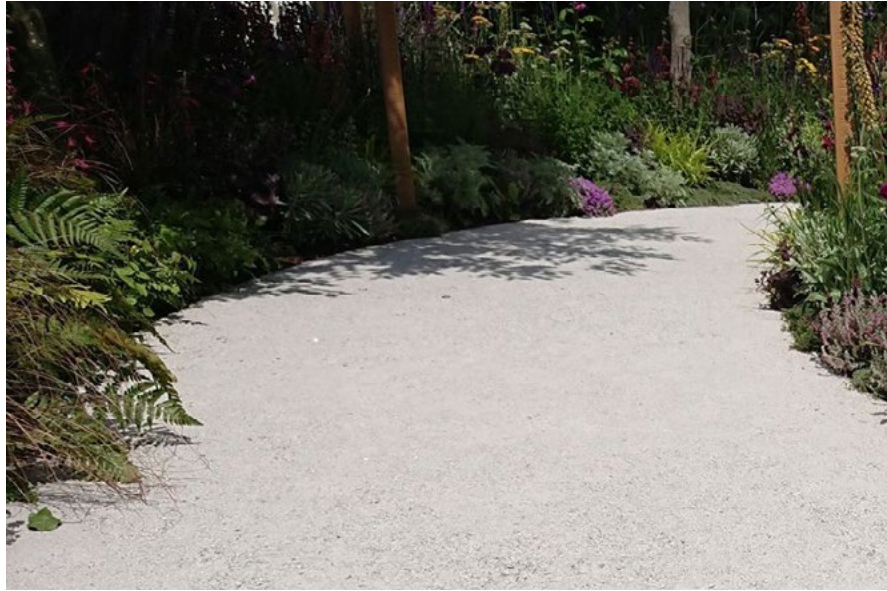
Self-binding gravel Colour: Buff Accessories: 3mm metal edging Buggy occasional vehicular overrun
