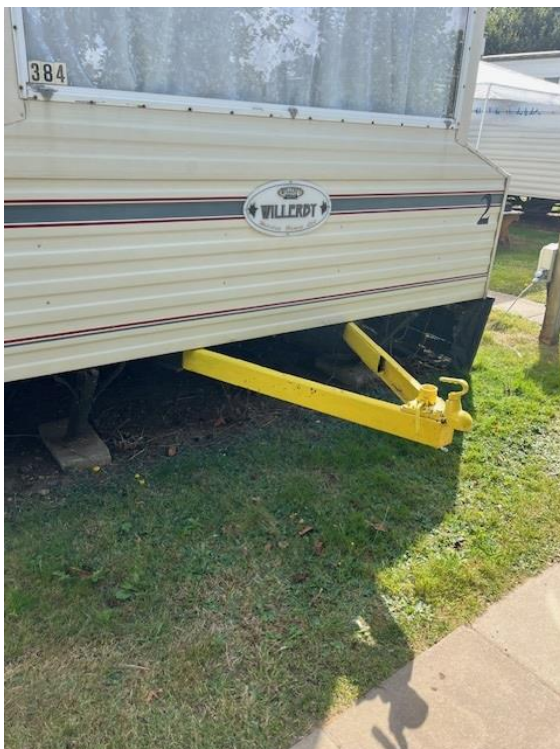
Photo.2 – towing hitch on mobile home
