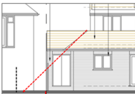
Figure 2 Vertical 45-degree angle test
