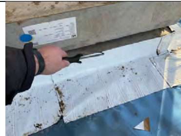
Stair Core. Probe testing along termination to the stair core base.
