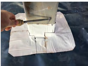
Probe testing a typical stanchion detail in the stair core area.
