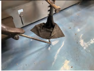
Probe testing to armoured joint pins.
