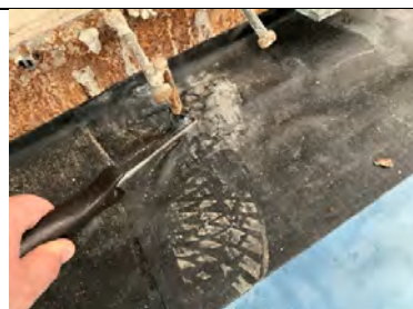
Probe testing armoured joint pins.
