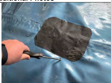
Probe testing installer CQA patch repairs.
