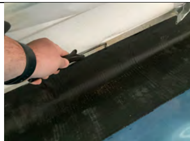
Probe testing along perimeter edge termination detailing.
