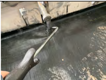
Probe testing to detailed armoured joint pins.
