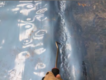
Testing to the lap joint.
