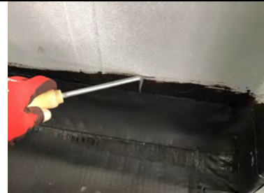
Probe testing a typical steel stanchion detail.
