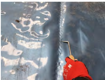
Probe testing a typical hand welded membrane lap.
