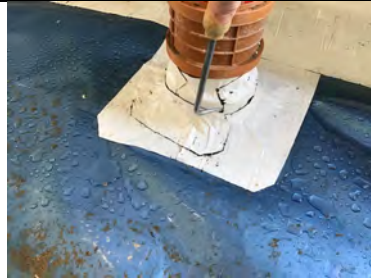
Probe testing a typical pipe penetration detail.
