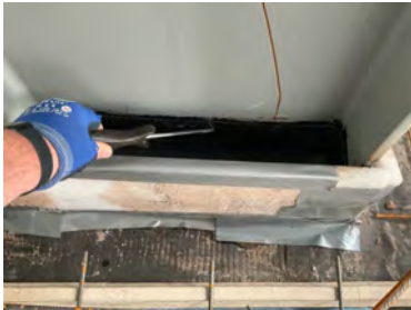
Probe testing to steel stanchion details.
