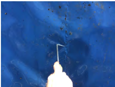
Probe testing a hand welded membrane lap in unit 3.
