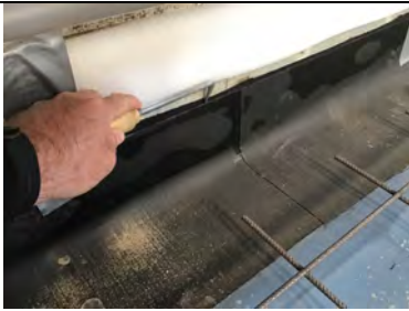
Probe testing the retro fit detailing around the perimeter of unit 6.
