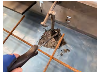
Probe testing to armoured joint pins.
