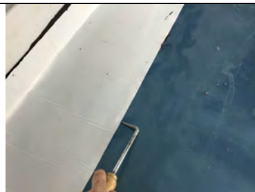
Probe testing the perimeter detailing.
