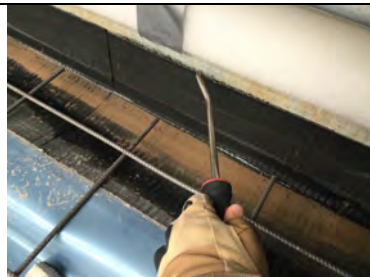
Testing to the JUTA GP1 SAM along the cladding rail.
