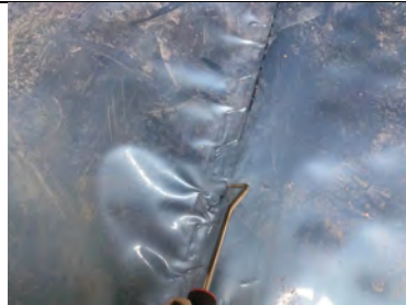
Testing to the welded lap joint.
