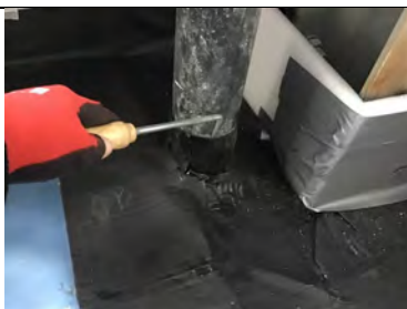
Probe testing a typical pipe penetration detail.
