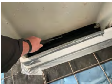
Probe testing to partially restricted steel stanchion.
