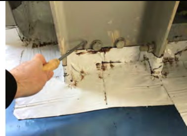
Probe testing a typical stanchion detail.
