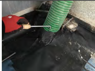
Probe testing a pipe penetration detail in unit 8.
