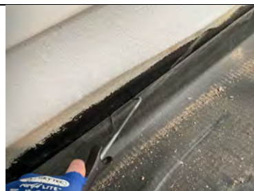
Probe testing along retrofit termination detailing to cladding rail.
