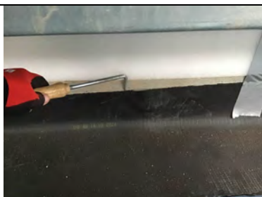
Probe testing the perimeter cladding rail detailing.
