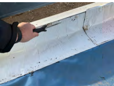
Stair Core. Probe testing along the perimeter cladding rail termination.
