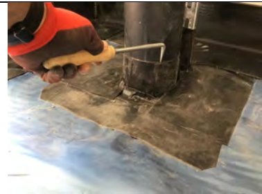
Probe testing a typical pipe penetration detail.
