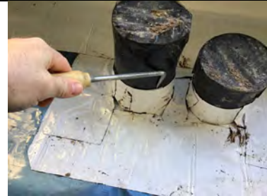
Probe testing a typical pipe penetration detail.
