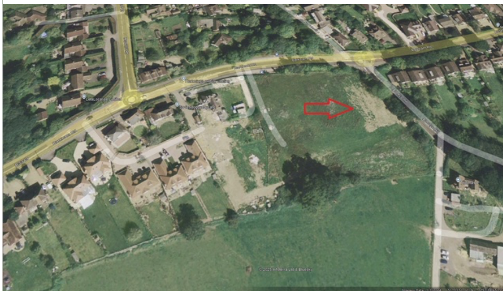
Figure 11: Imagery from January 2004 Shows a Bare Reinstated Patch in the Eastern Area Consistent with Backfilling
