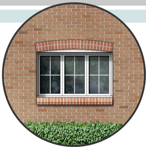
Split Coursed Brick Arched Headers With overhanging angled brick sills
