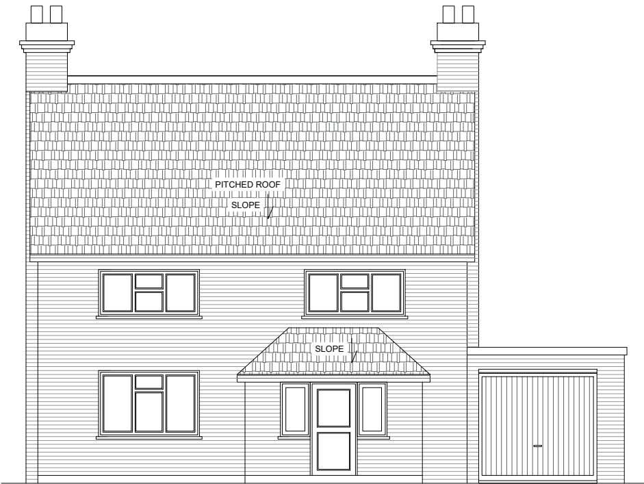
EXISTING FRONT ELEVATION
