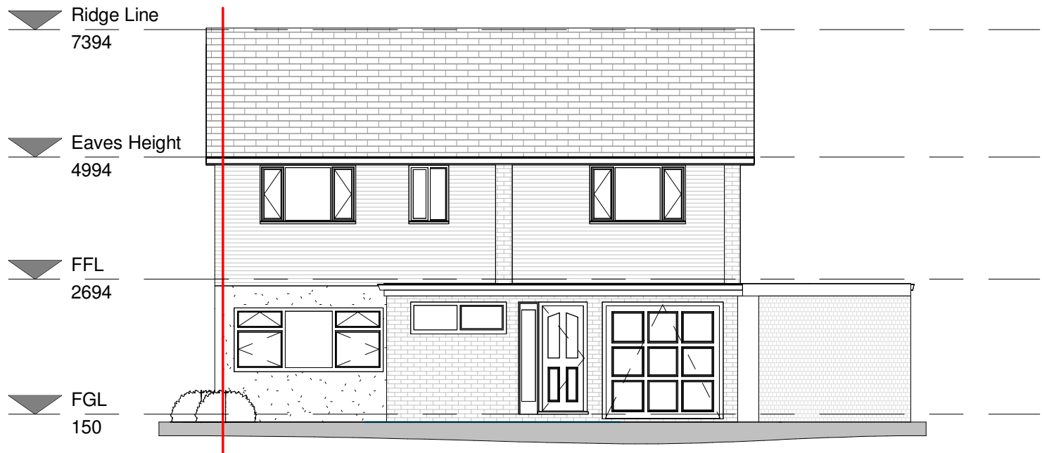
Existing Front Elevation 1 : 100
