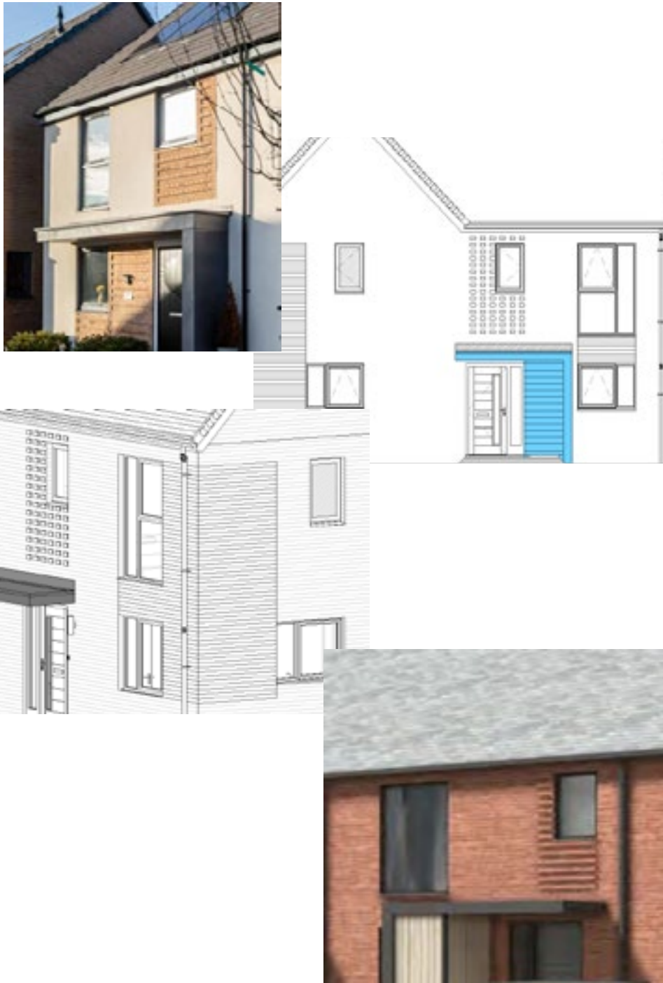
Projecting contrast brick feature as surrounds to windows on major elevations.
