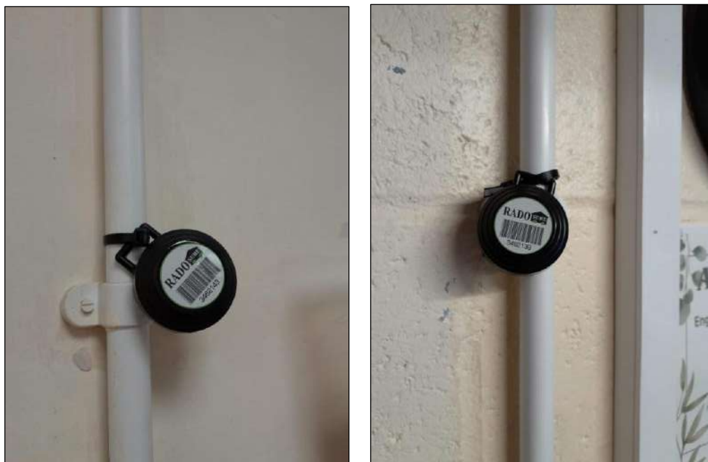
Figure 3 Selected GGS site photographs of the passive radon detectors deployed on site.
