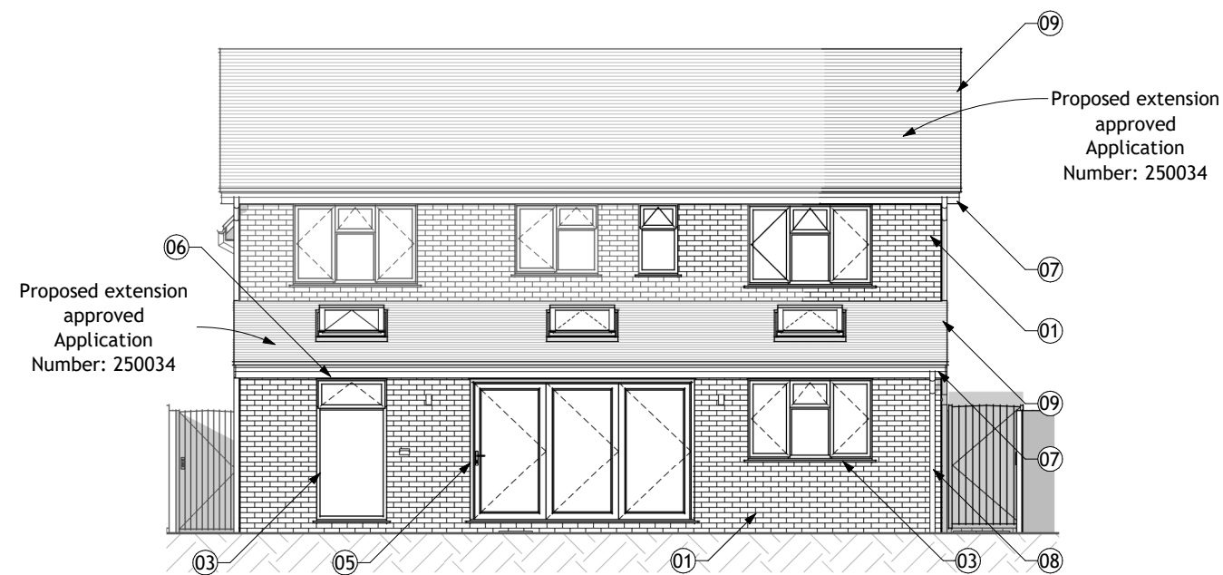
Proposed Elevation - East General Arrangement | Scale 1 : 100
