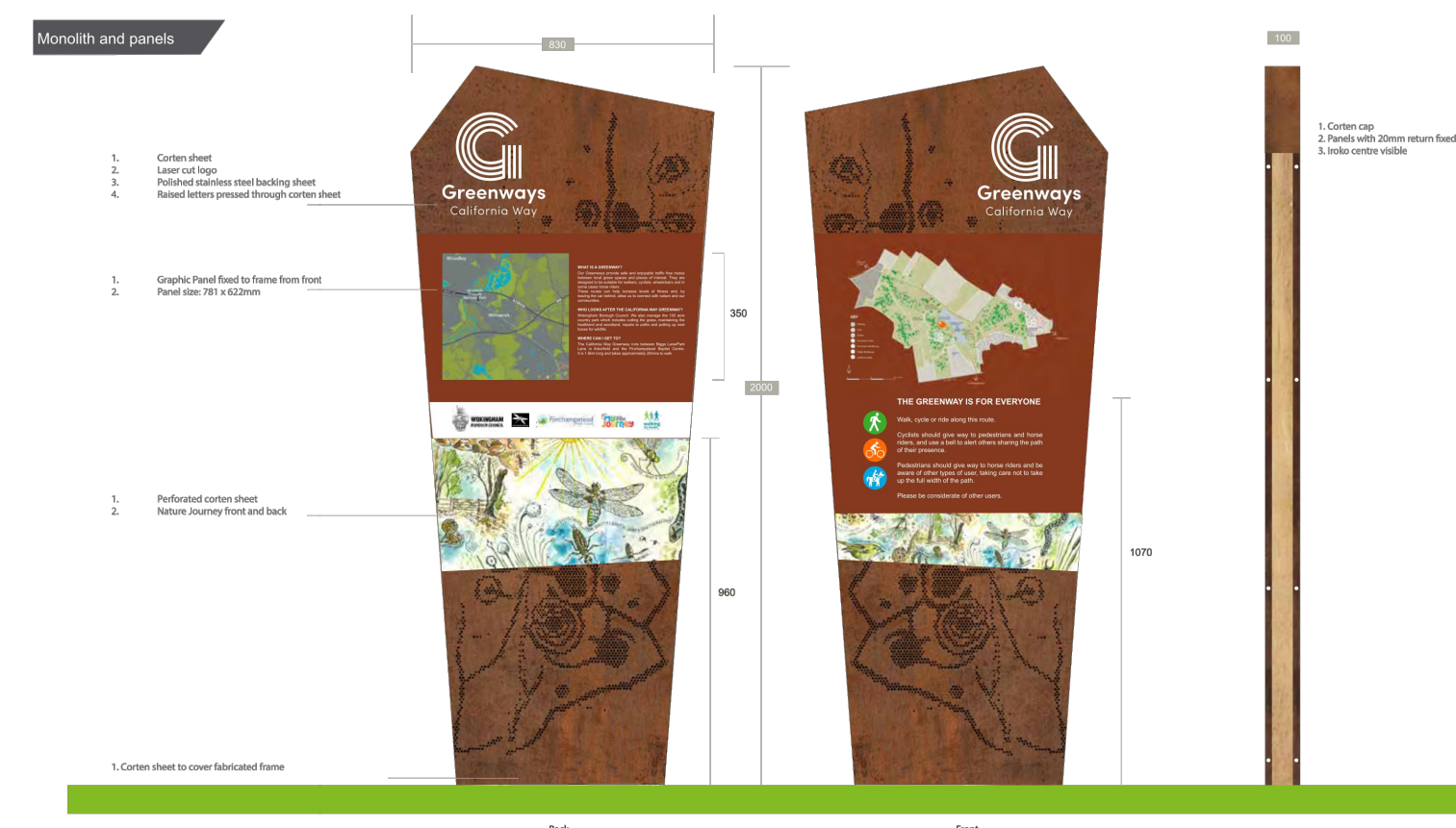
29 TYPE B.2 WAYFINDING SIGN ELEVATION SCALE - 1:20 @ A1 & 1:40 @ A3
