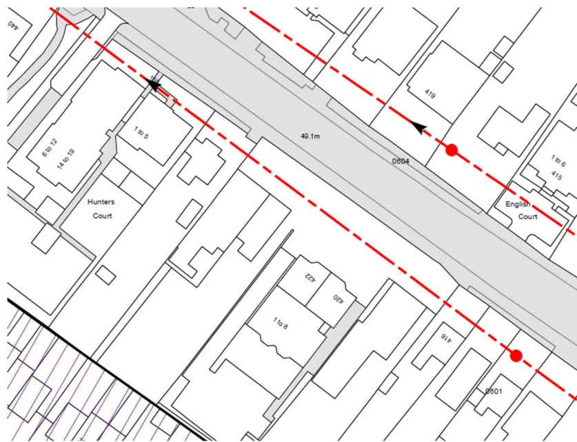
Figure 2: Extract of Thames Water's Sewer Map
