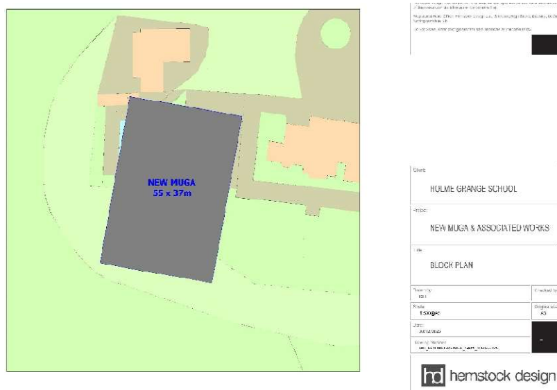
Block plan showing the new MUGA footprint abutting but not encroaching on the shingle path
